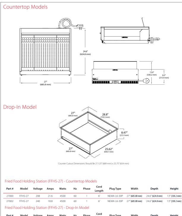
Part # Model Voltage Watts Hz Phase Width Amps Plug Type Depth Height Length 6' 27" (685.80 mm) 24.6" (624.8 mm) 13" (330.2 mm) 27017 FEHS-27 208 18.8 4500 60 1 NEMA L6-30P
