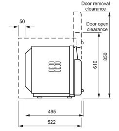
Allow a minimum of 50mm clearance to sides, top and rear to allow air to circulate freely
