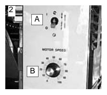
Turn on Motor Power Switch (A) and set Motor Speed Control (B) to desired setting. (Use a setting of "50" to start.)
