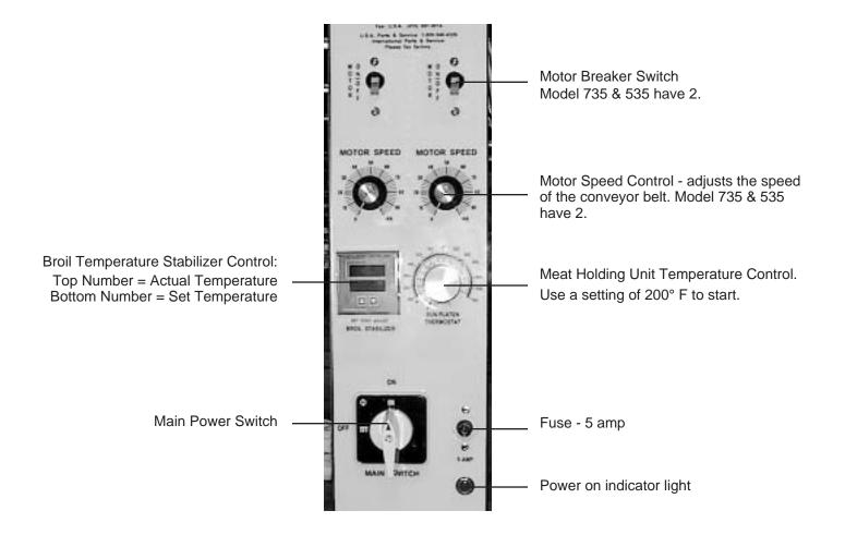
After the hamburgers are cooked, they drop into the Holding Unit, which uses an electrically heated base to maintain a set temperature for holding the hamburgers or chicken.
