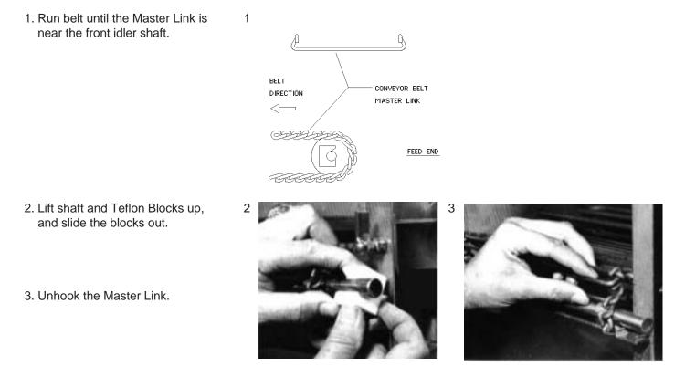
To reassemble, reverse the procedure. Be sure to reassemble the belt with the knuckle opening facing away from the direction of travel.
