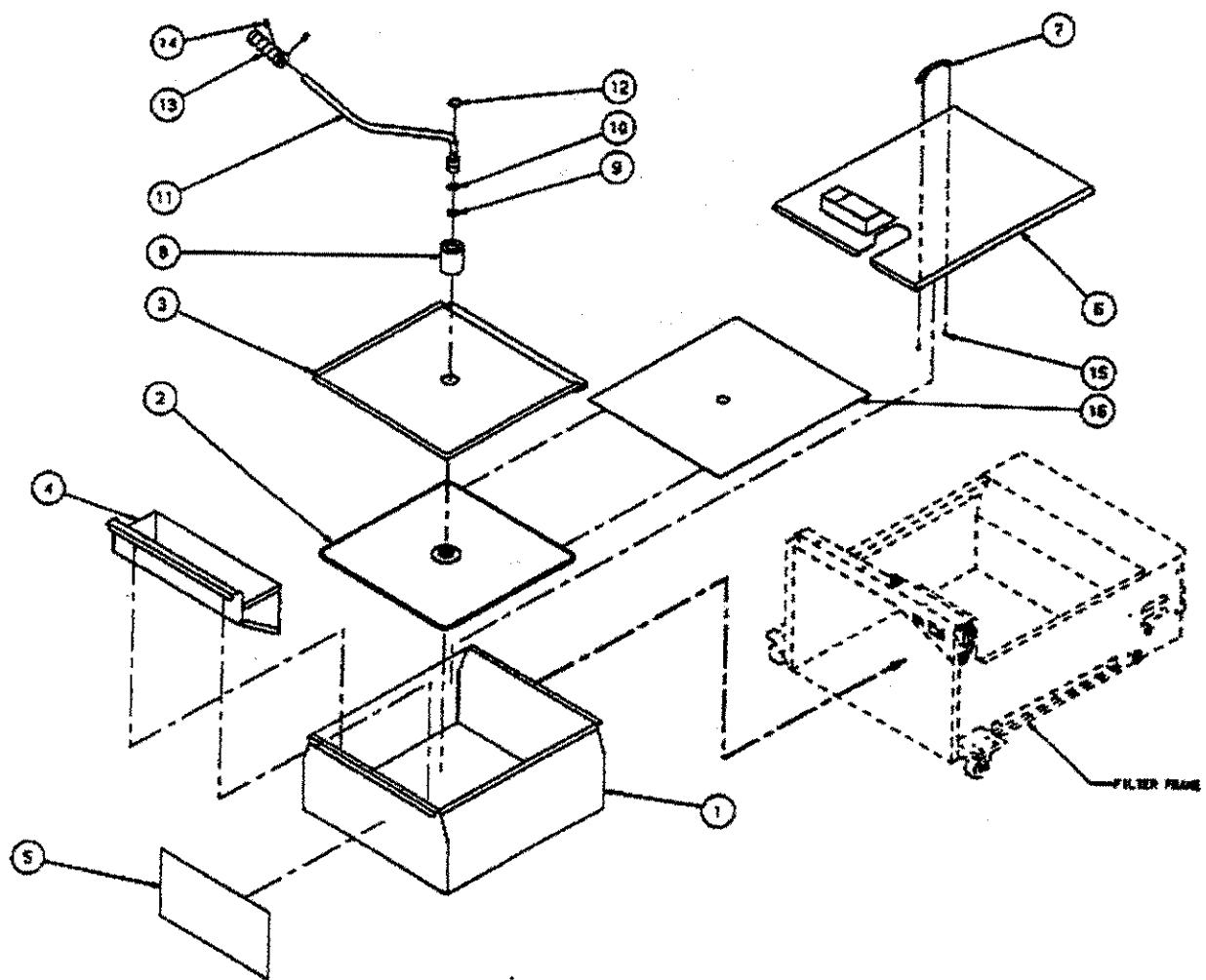
Figure 5-5 UFM Filter, Pick-Up/Pan Assembly
