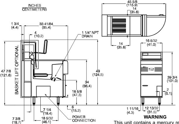
NO POWER CORD IS SUPPLIED WITH THE UNIT. ELECTRIC SERVICE MUST BE HARD WIRED BY A LICENSED ELECTRICIAN!
