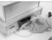
To insert the new tube, first insert the top end through the hole that leads to the platen. The tube will fit through the insulating bushing
