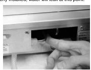
Using pliers, gently pull the tube out from the platen. You may need to softly rock it back and forth. Replace the black insulating bushing if the original bushing pulled out with the water tube. All units must have a bushing installed. To reinstall the bushing, lubricate it with water and push it back into the opening.
