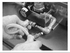
Connect the longer end of T-Connect to the steamer whose regulator is farthest from the inlet water line. T-Connect's female end to steamer's male end.
