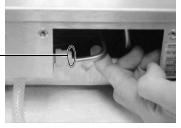
Push the other end of the tube into the water valve. Ensure that you feel it click into place. Gently tug on the water tube to check if it is secure. If the tube slides out, reinstall the tube. If tube is improperly installed, water will leak at this point.
