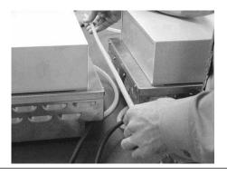
Connect the inlet water line's female end to the T-Connect's male fitting. The two steamers have been connected to the inlet water line. Set both steamers' regulators to 25 psi.
