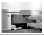
To pull the tube out from the water valve, push in the grey disk on the water valve and then slowly slide the tube from the water valve.
