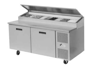
ELECTRICAL: The units will be provided with a 8' power cord and 3-wire grounded plug as standard, pre-wired for 115 volt, 60 hertz, single phase operation. Export voltages are available and require hard wiring in the field to the units main junction box, (unit will be shipped on legs for export applications, unless specified otherwise).
