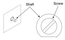
Calibrate the thermostat by holding the shaft in place while turning the screw counterclockwise to increase the temperature. or clockwise to decrease the temperature. Figure 21 -
