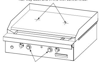
Each knob is attached to a thermostatic valve located behind the valve panel.
