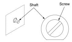
Calibrate the thermostat by holding the shaft in place while turning the screw counterclockwise to increase the temperature. or clockwise to decrease the temperature. Figure 23 -
