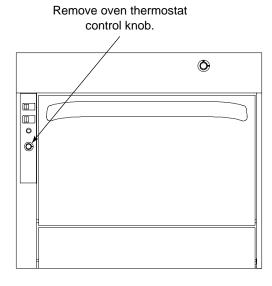
With the control knob removed, the control shaft will extend out of the control panel.
