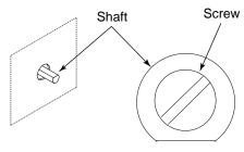
Calibrate the thermostat by holding the shaft in place while turning the screw counterclockwise to increase the temperature, or clockwise to decrease the temperature.
