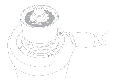
Scotsman grease needle pn 02-3559-01 and Scotsman bearing grease cartridge, pn A36808-001. Be sure to inject grease evenly and thoroughly.
