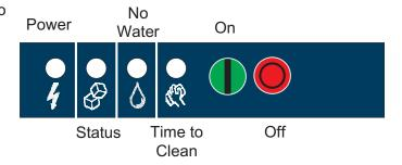
There are four indicator lights at the front of the machine that provide information on the condition of the machine.
