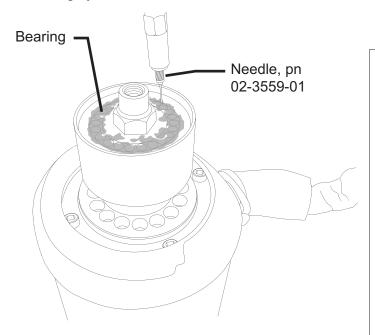
If the grease is uniformly white, no further action is needed. If very gray, rusty, wet or has any embedded metal, have the bearing replaced.
