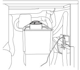
Removing the water shed & unscrewing the breaker cover (left hand threads).
