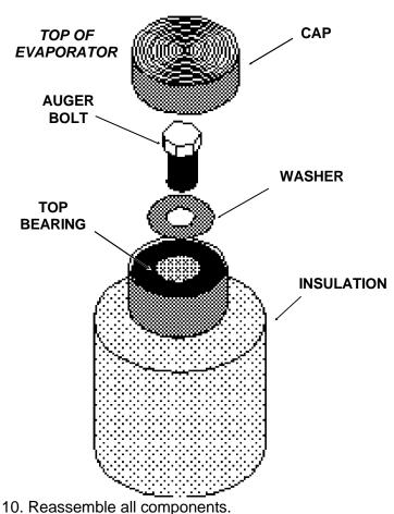
Ice Breaker and Auger Removal for Inspection
