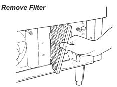
4. Wash the surface of the filter off with cold water, or, if torn or so dirty it can't be cleaned, replace with a new filter.
