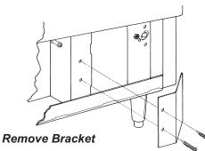
3. Pull the filter forward and twist it slightly to pull it though the slot in the front base of the ice machine.
