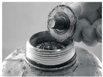
Thrust Washer and Bearing
