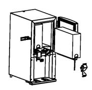
Pull dispensing tube out of valve and remove product box from cabinet
