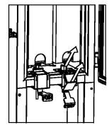
Tilt valve insert assembly forward and pull up and out at an angle
