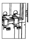
Replace valve insert assembly and be sure it snaps into place.
