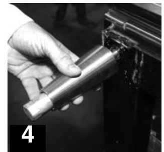
4 Thread leg into cabinet bottom frame rail.
